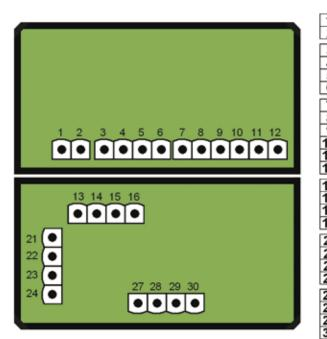
1 2 -VDC +VDC Power Supply NO COM 3 SSR1 4 5 6 NO COM SSR2 7 8 9 10 11 12 NO COM NC RELAY1 NO RELAY2 COM NC 13 +V 14 15 FREQ IN DIR Flow Sensor 2 16 GND 21 -LOOP2 22 +LOOP2 23 -LOOP1 24 +LOOP1 Analog Output 27 28 29 30 +V FREQ IN DIR Flow Sensor 1
